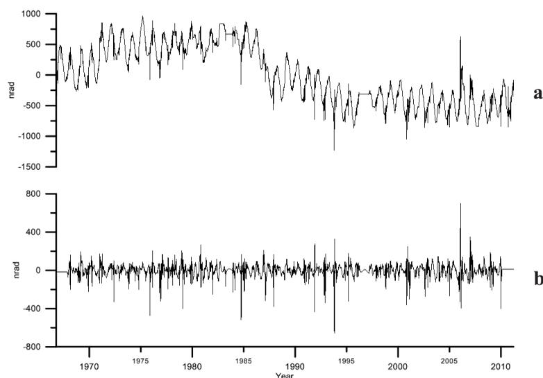
Fig. 6 - The E-W component before and after the signal processing for the time interval October 13, 1966 to March 22, 2011: a) original recording; b) the signal used for the study.
