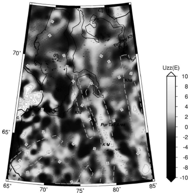
Fig. 2 – Gravity tensor component  $T_{zz}$  (Eötvös) for the Pur Taz area, a central segment of the West Siberian Basin. This gradient component enhances the presence of the proposed graben-rift structures. Geographic features as in Fig. 1. Tensor derived from potential field model EGM2008 (Pavlis et al., 2008).
