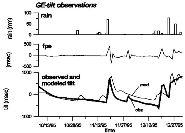
**Figure 2.** Modeling of the hydrologically-induced tilt signal at GE-station. Observed tilt records have been reduced to daily sampling and long period signals have been removed. Rainfall, forward prediction error of modeling (fpe) and modeled (light trace) and observed (heavy trace) hydrologically-induced deformation of tilt are shown.
