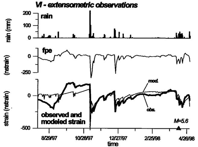
**Figure 4.** Extensometric records at station Villanova for the period Nov. 1, 1997 – Apr. 30, 1998. The onset time of the Slovenian  $M = 5.7$  event is April 12, 1998 (black triangle). The coseismic step has been taken out. Rainfall, forward prediction error of modeling (fpe) and modeled (light trace) and observed (heavy trace) hydrologically-induced deformation of tilt are shown.
