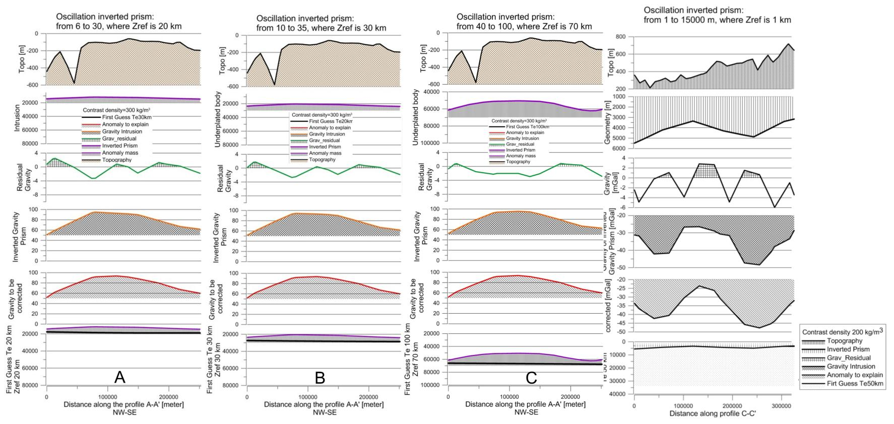
Fig. 10 Inverse modeling in the northern Angola basin. The model simulated in A: a mass intrusion, in B an underplating between crust and mantle, the Zreference is respectively: 20 and 30 km, and the contrast density is  $300 \text{ kg/m}^3$ . In C the model simulates a mantle densification.
