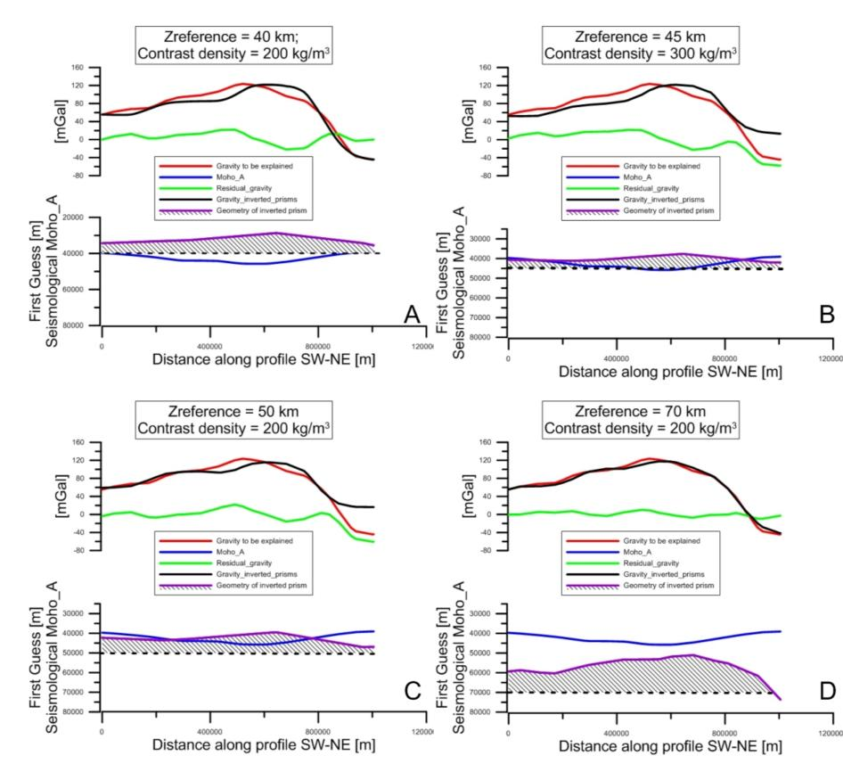
residual Bouguer Fig. 8 The anomaly, where the first guess is the Moho of Assumpção et al. The prisms define the (2013). density anomaly body. Reference depth (Zref.) is 40 km
