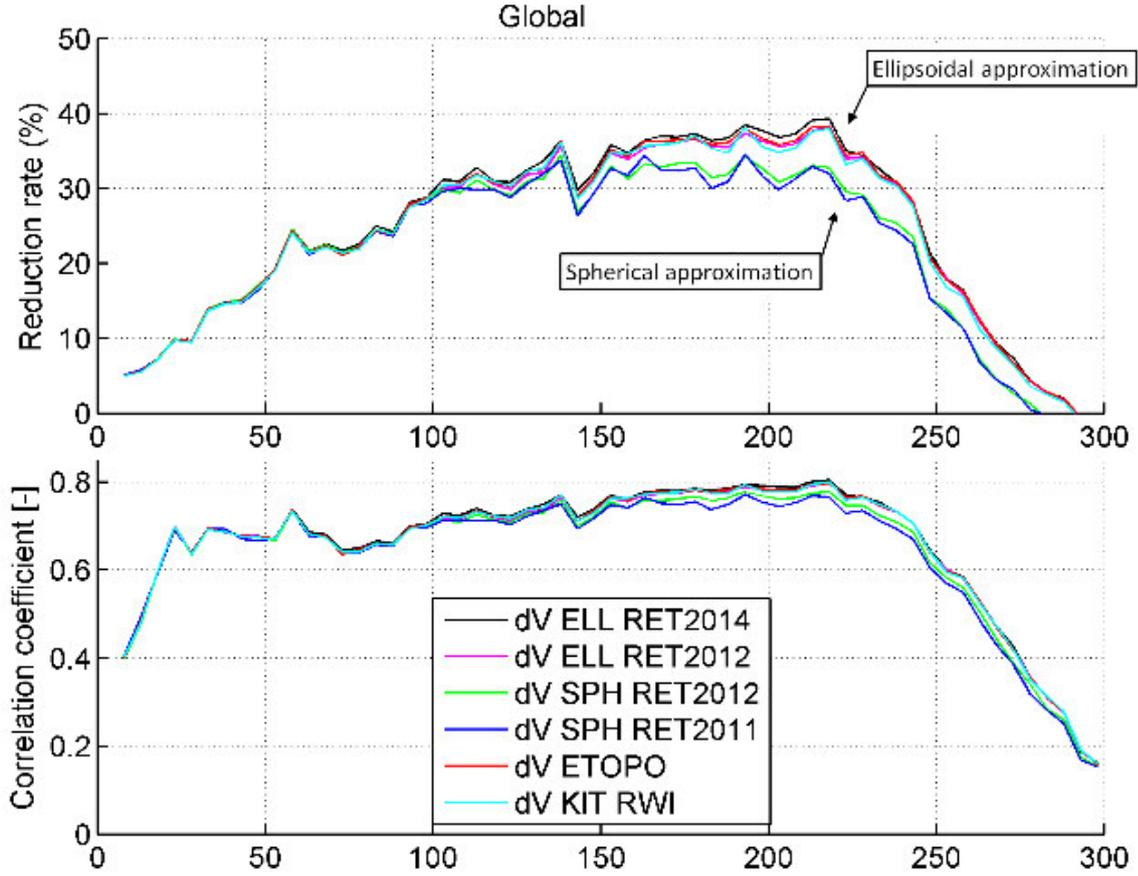
Figure 2 : Evaluation of different topographic data sets and their respective topographic potential models w.r.t. the model *GO\_CONS\_GCF\_DIR5* in terms of reduction rates (upper plot) and correlation coefficients (lower plot).
