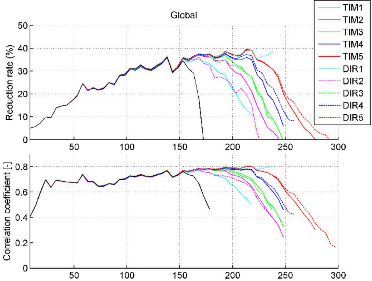
Figure 1 : Evaluation of 5 generations of ESA GOCE models from the time-wise method (TIM: solid lines) and the direct method (DIR: dashed lines) using the topographic potential model  $dV\_ELL\_RET2014$ . Black ITG-GRACE2010S.
