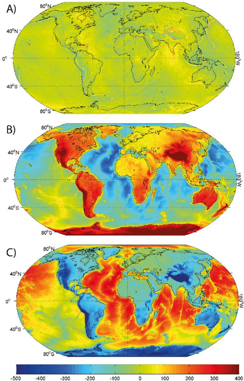
Figure 3: Global maps of gravity disturbances from a) the ESA GOCE gravity model  $GO\_CONS\_GCF\_TIM5$ , b) the topographic potential model  $dV\_ELL\_RET2014$  and c) derived Bouguer gravity anomalies ( $c=a-b$ ) at an evaluation height of 10 km; models are truncated at degree 250 (units are mGal; Robinson projection).
